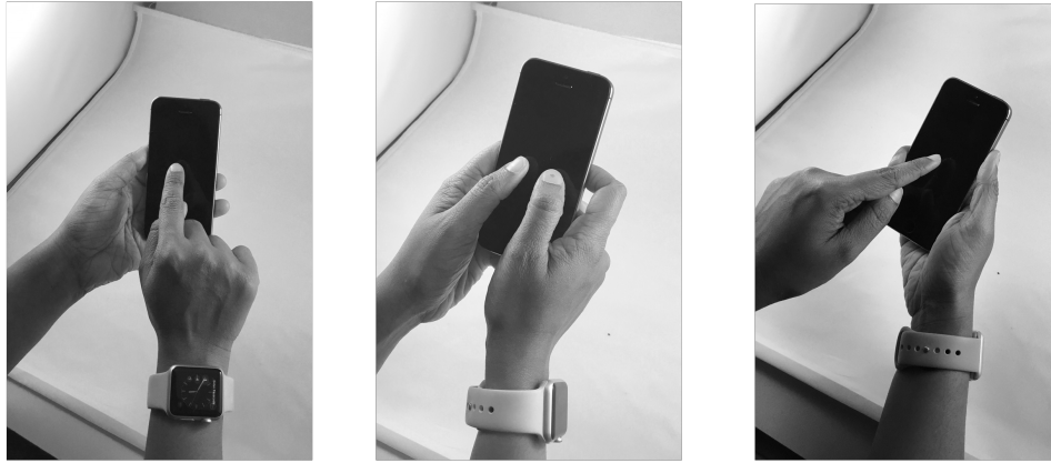
Figure 7.2: Wristband orientation in three grips. From left to right: NW (phone held in non-wristband-hand and input with wristband-hand), BB (phone held with both hands), and WN (phone held in wristband-hand and input with non-wristband-hand).
