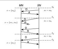
Fig. 3 Adaptive security at work (D = data, A = ack, R = reissue)
